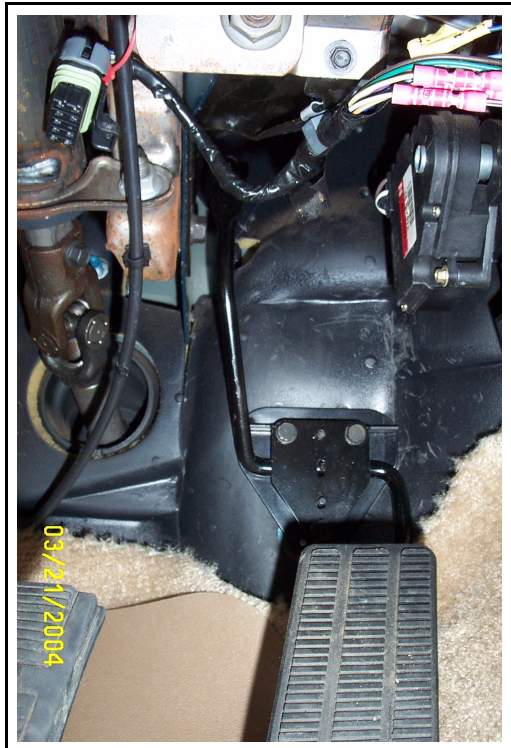
Throttle pedal bolts right in place of APP. APP connector is tied up out of the way. Splices in APP wires are left over from failed experiments!
