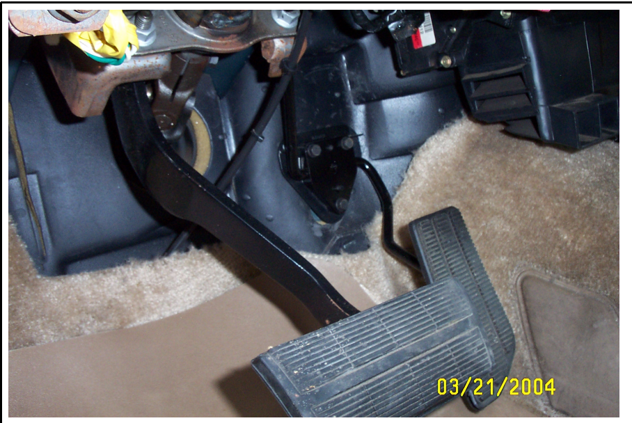
No APP mods required here! Throttle pedal from a gas engine truck looks right at home.
