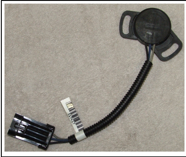
Throttle position sensor (TPS) installs on the DB2 pump. Slots allow adjustment as noted in text.
