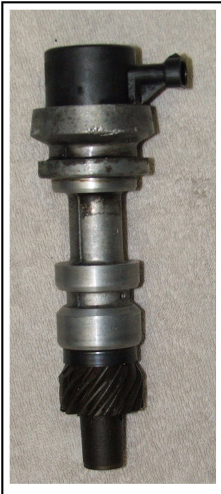
Engine Speed Sensor (ESS) replaces your existing oil pump drive.
