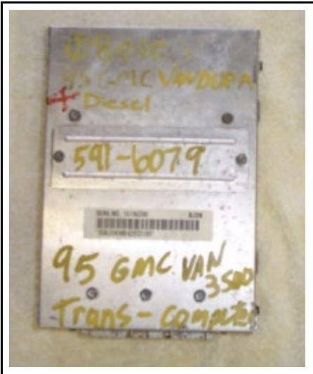
The GM 4L80E transmission computer (TCM)
